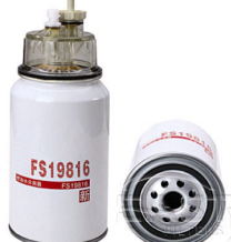
Fuel Filter FS19816 with bowl EF-42056
